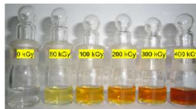
Fig.8. Pictures of pre-and post-irradiated [EMIM][FAP] RTIL. A similar color appearance was observed in the case of [EOHMIM][FAP]. Reproduced from Ref. [29] with permission from the Royal Society of Chemistry.
